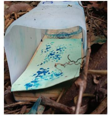
Tracking tunnel constructed of plastic and wood at the base. Mongoose paw prints are visible on the green tracking card
