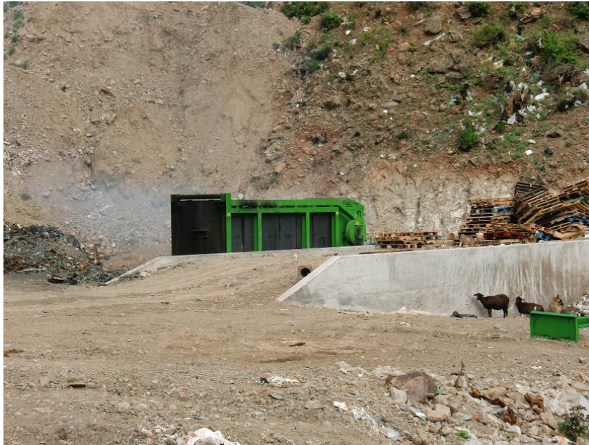
Figure 22. Open air burner of the Saba landfill in operation. (Photo A. Debrot).
